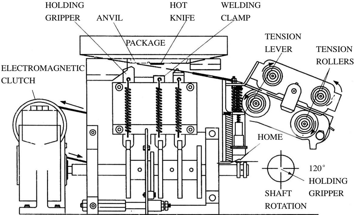
FIGURE 16. HOLDING GRIPPER AND HOT-KNIFE
