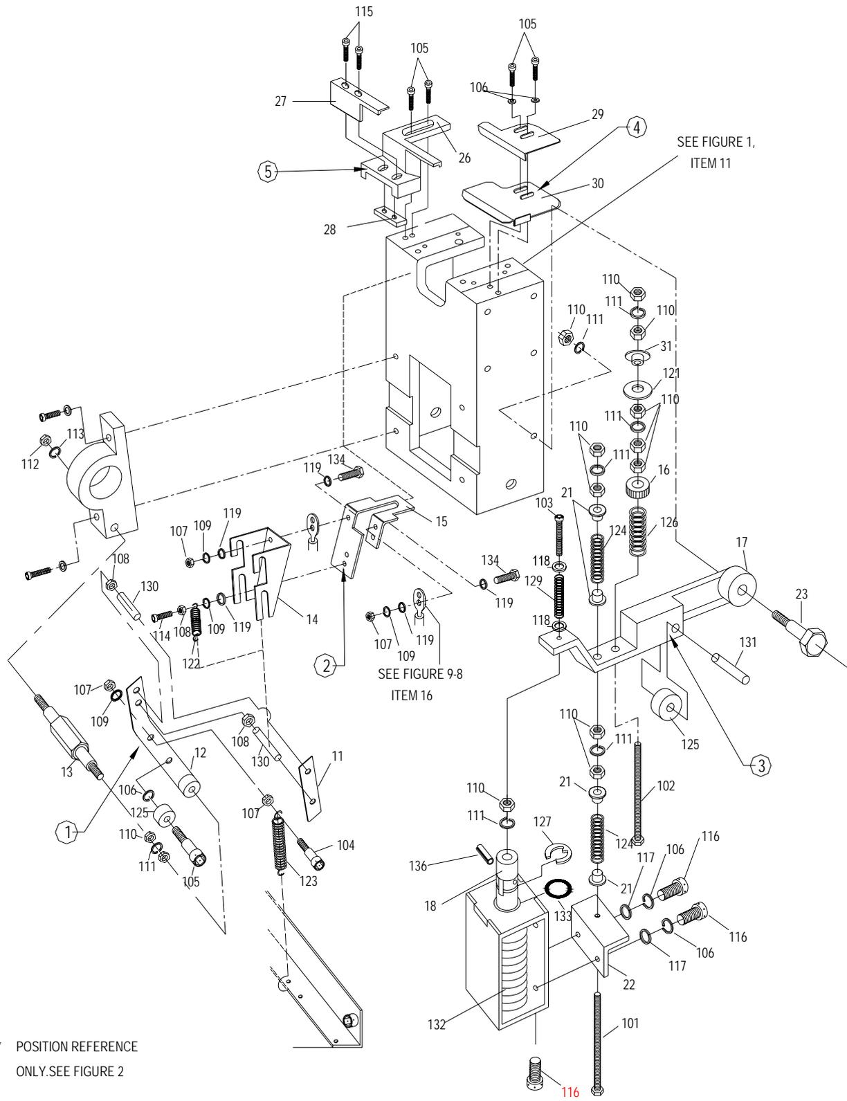
FIGURE 5.HOT-KNIFE AND TENSION LEVER ASSEMBLIES
