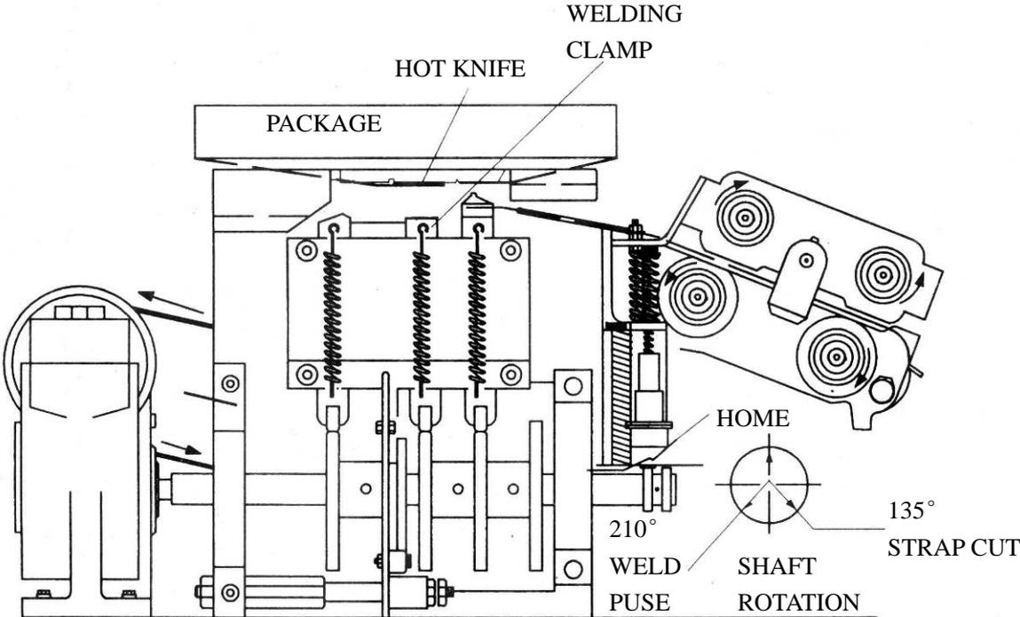
FIGURE 17. STRAP IS CUT & WELD IS MADE
