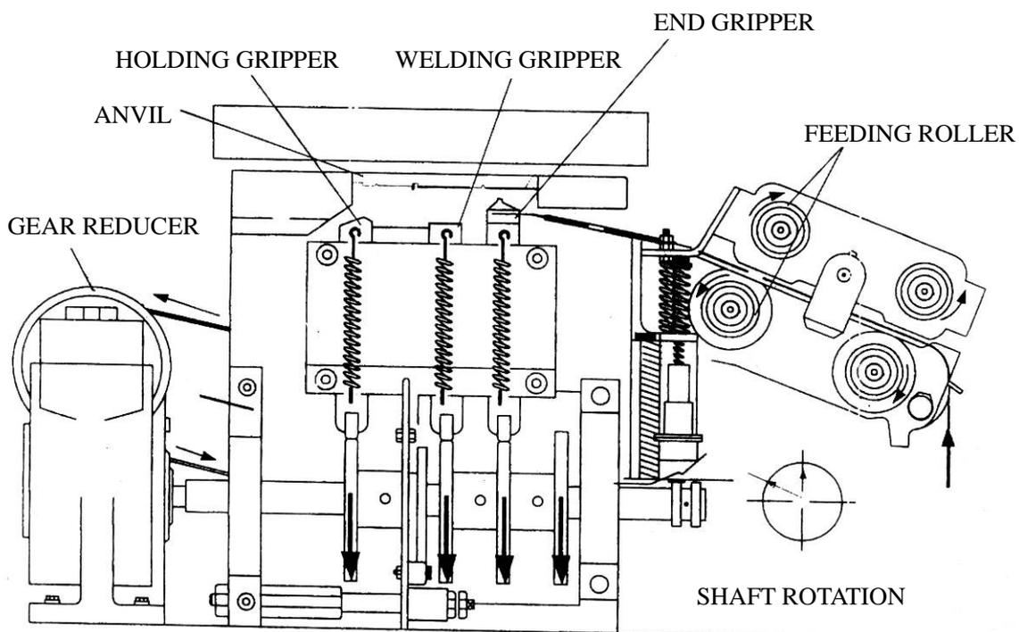
FIGURE 18. WELDING STRAP IS RELEASED;
