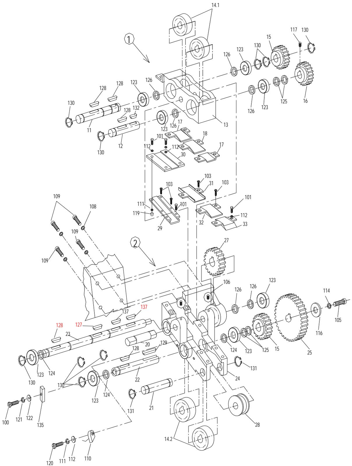
PARTS LIST, FIGURE 4 TENSION ADJUSTMENT AND SENSING ASSEMBLIES
