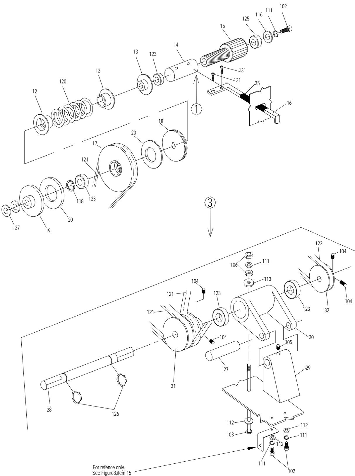
PARTS LIST, FIGURE 5 HOT-KNIFE AND TENSION LEVER ASSEMBLIES
