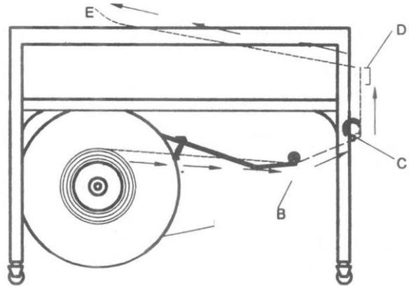
FIGURE 9. STRAP THREADING DIAGRAM
